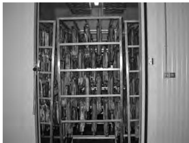
Figure 18.5. Example of a fermentation/drying chamber with computer control of temperature, relative humidity, and air rate. (By courtesy of Embutidos y Conservas Tabanera, Segovia, Spain.)
