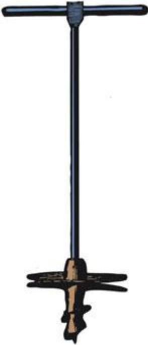
• A hole borer lifts the soil from the hole without having to use spades. These borers can be used by hand or electric models can be purchased for the same purpose.
