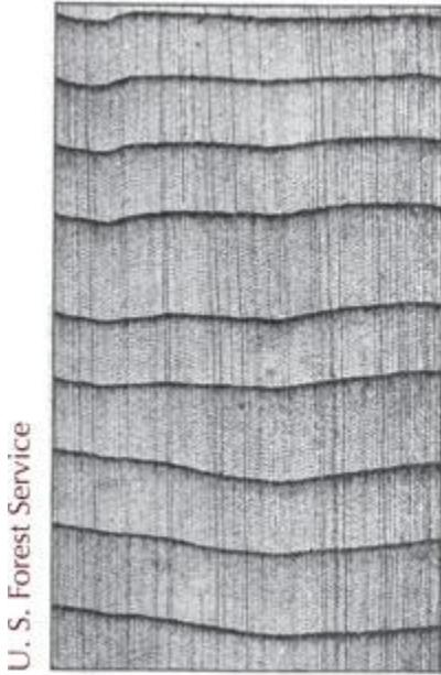
▲ Fig. 69. Wood of arbor vitæ as seen through a microscope. The wood is light and, like that of other evergreens, is non-porous and uniform in texture.
