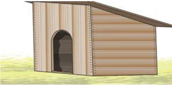
▲ This kennel has a floor that is 2 feet square, is 3 feet 4 inches high in front, and the roof has an overhang of 8 inches.
