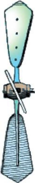
• Each spoke should be cut at an angle so that the blades will have the pitch to make the wind turn them.
