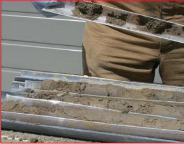
▲ To determine the various layers of your soil, called your “soil profile,” a core sample can be taken. This requires a boring machine, which will insert a hollow core rod, or “probe” like these shown here deep into the ground to extract soil. The layers will be distinguishable by the change in soil color. Several core samples can be mixed together for a more accurate soil test.
