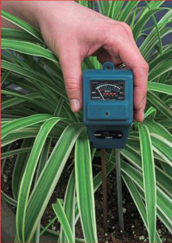
• This electronic soil tester runs on one AA battery and gives pH, nutrient, and moisture level readings within minutes.
