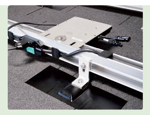
ABOVE: Rails with channels offer the cleanest installation. The channels are open at the top but are almost entirely covered by the modules.
