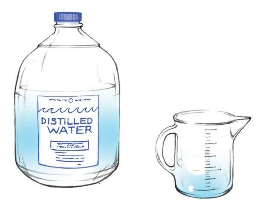
ABOVE: Distilled water and a paper cup or a glass with a spout (for watering batteries)
