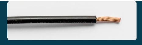
CHARACTERISTICS: Single-conductor, insulated wire for outdoor exposure. Rated for 90°C (184°F) for wet and dry locations. Solid or stranded copper, copper-clad aluminum, or aluminum conductor. UV-protected sheathing.
